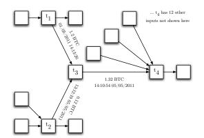
Fig. 2. An example sub-network from the transaction network. Each rectangular vertex represents a transaction and each directed edge represents a flow of Bitcoins from an output of one transaction to an input of another.
