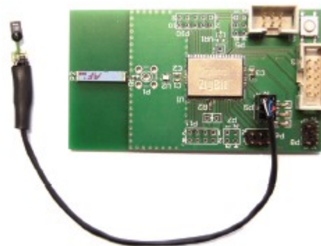
Figure 3 The Pixie node is a flexible prototyping platform which is equipped with extension headers for external peripherals.
